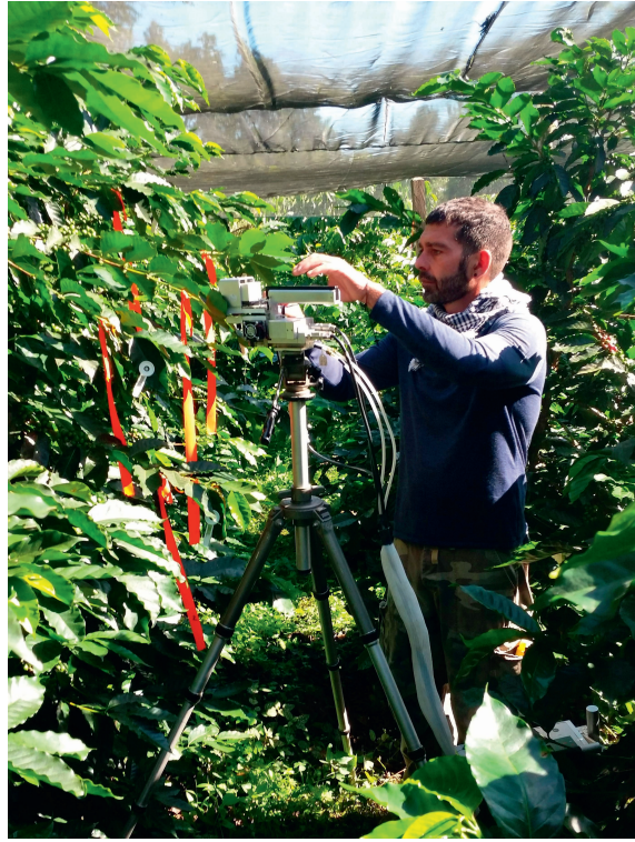
Photo 9.2. Measurements of photosynthesis on hybrid varieties of C. arabica cultivated under shade simulating agroforestry conditions (Teocelo, Veracruz, Mexico). © Luc Villain/CIRAD.
