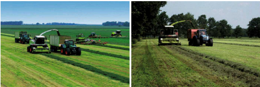
Grass harvesting for silage. Left: Demonstration of machinery types. Right: Self-propelled forage harvester filling a wagon pulled by tractor. Source: ILVO – Merelbeke.
