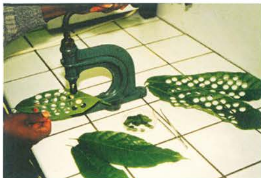
Preparing leaf discs with a mechanic cork borer.
