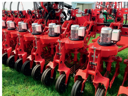
Figure 6.1. Detail of an Eco-Mulch inter-row shredder (Eco-Mulch and Arvalis, 2019) (photo: C. Huyghe).
