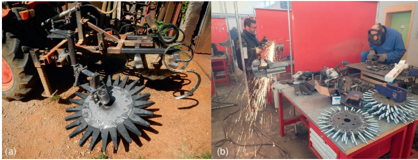
Figure 6.2. Hoeing star designed at Atelier Paysan for mechanical weeding in vine rows; (a) model of a hoeing star that can be easily adapted to different mounts; (b) stars being made during a training session at Atelier Paysan (L'Atelier paysan, 2021).
