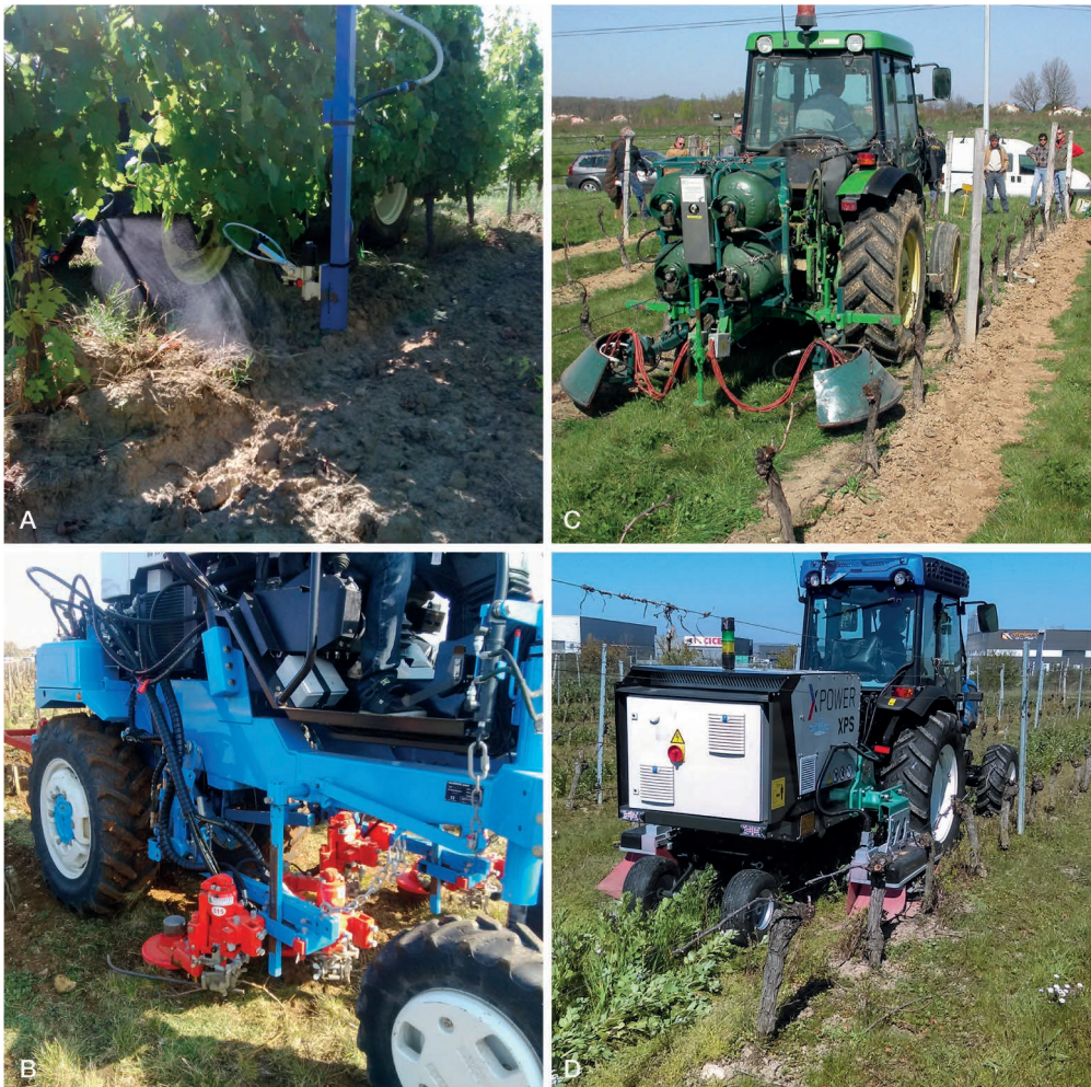
Figure I-6-2. A: application of herbicides under the row; B: rotary tillers mounted on a straddle tractor; C: propane-powered thermal weeder; D: electric weeder prototype. © Christophe Gaviglio, IFV81.
